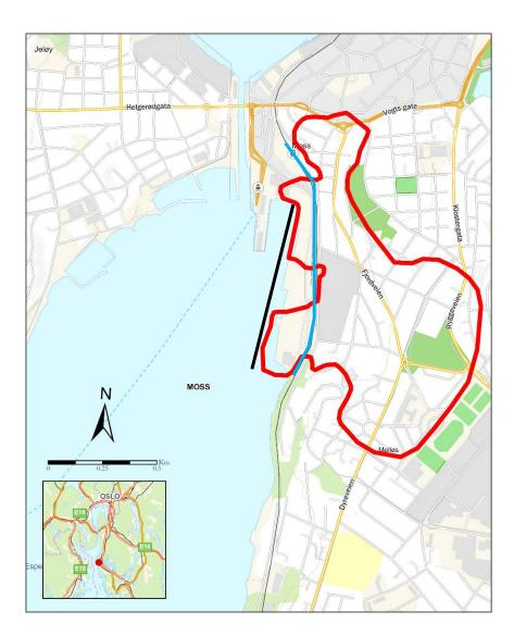
Figure 2-1 Quick clay area (red line), landslide foot scenario one (blue line) and landslide foot scenario two (black line). Inset shows location of Moss (red dot), south of Oslo.
